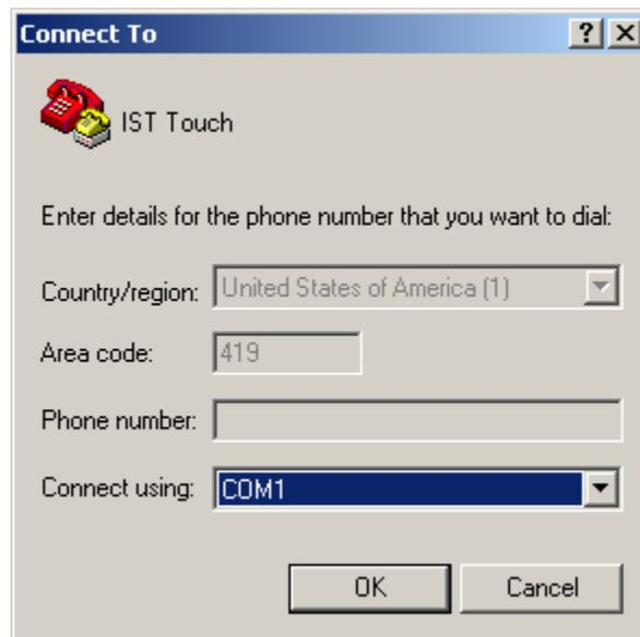
COM1 is the default RS232 port but if you are using a USB adapter you may need to check you port settings to see which port the Touch Panel is connected to.
